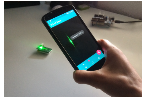
Figure 1: Aiming the VLC board with his smartphone, the user is getting the ambient temperature
